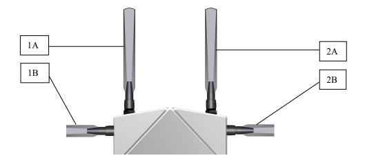
The AWK-6232 supports 802.11 a/b/g/n with 2x2 MIMO technology and dual RF redundancy. Antennas 1A and 1B are the MIMO antennas associated with RF1, and 2A and 2B are the MIMO antennas associated with RF2.
